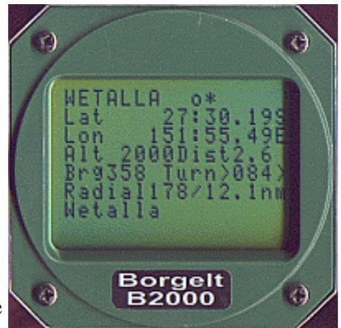
You can enter up to 10 **USER turnpoints**, using this page (1 to 9 then 0). This allows correction of an incorrect turnpoint in the database by replacement by a user point or quick addition of a turnpoint temporarily. These points are NOT added to the permanently stored database but are in Super Capacitor backed RAM where they will stay for a week or two. This prevents corruption of the database by casual use.
