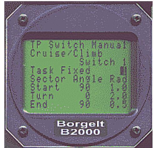
The next selection is the task type. Up to 10 different named task types can be uploaded from the B2000User program. These fall into three classes.
