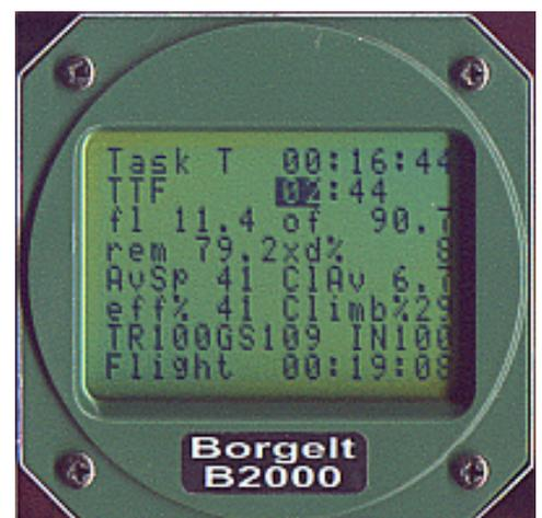
The **FLY TO** page gives the same information as the **GRAPHIC** page but in alphanumeric format and with greater resolution. The name of the turnpoint you are flying towards is shown. The final leg is warned by a FIN LEG appearing next to the wind component information. Most of the time the **GRAPHIC** page will be sufficient to make decisions and get a snapshot of the navigational and final glide situation to without spending excessive time looking in the cockpit.
