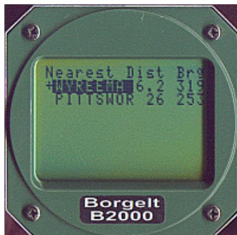
change batteries or return to manufacturer for service. Memory backup is by Super Capacitor. This is good for about 10 hours at least(usually much longer- some weeks), so after entering a task after briefing you can turn off the instrument and when about to launch turn it on again with the planned task preserved.
